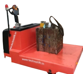
Die / Mould Platform Battery Operated Truck Capacity - Up to 12,000Kgs
