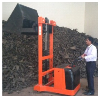
Counter Balance Bucket Stacker Capacity - up to 2000Kgs Lift height - Up to 3000mm
