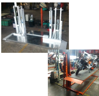
Lifting Platform - Bike Tilting Capacity - 500Kgs Lift height - 1000mm
