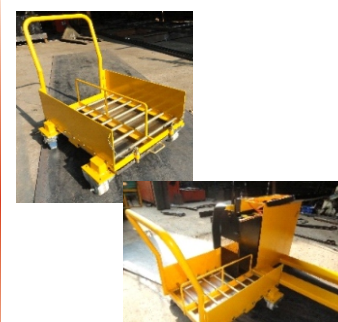
Battery Changing Trolley Capacity - Up to 1500Kgs
